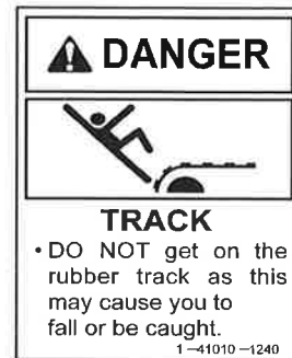
(10) Beware of rotating crawlers (2 locations, left and right) (1-41010-1240)
