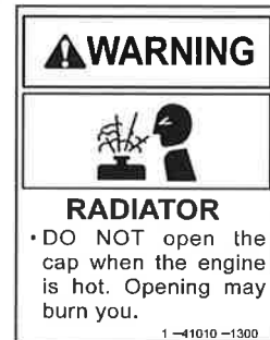
(12) Beware of high-temperature coolant (1-41010-1300)
