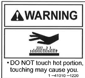
(13) Beware of high-temperature muffler (1-41010-1220)
