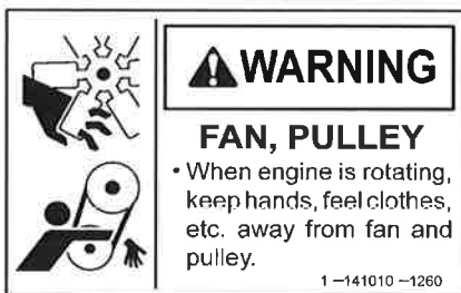
(11) Beware of rotating fan and pulley (1-41010-1260)
